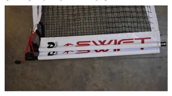
Note the tangle of the red cord because the cord was not properly tucked into the vinyl wrap before rolling.
